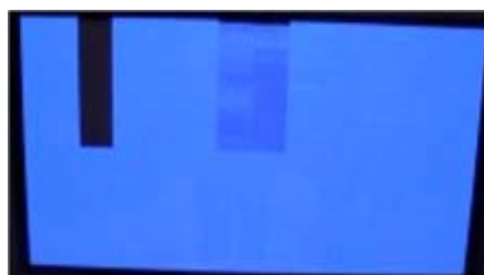
The defect area is not as wide as the ribbon cable from the buffer board.
