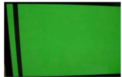
The defect area is not as wide as the ribbon cable from the buffer board.
