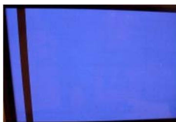
The defect area is not as wide as the ribbon cable from the buffer board.
